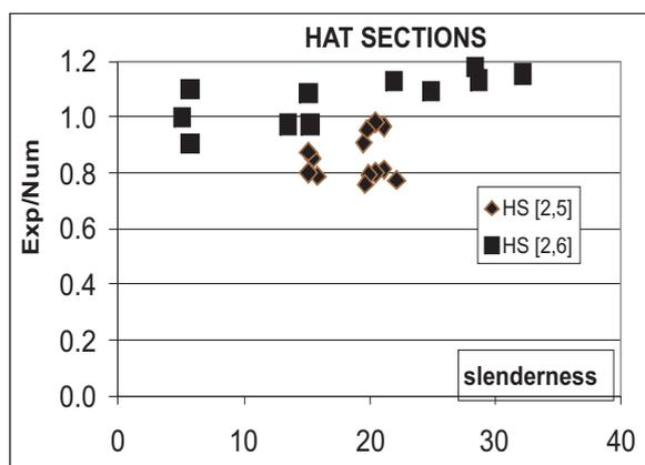
Figure 3 - Accuracy of the method for hat sections: error versus the specimen slenderness
