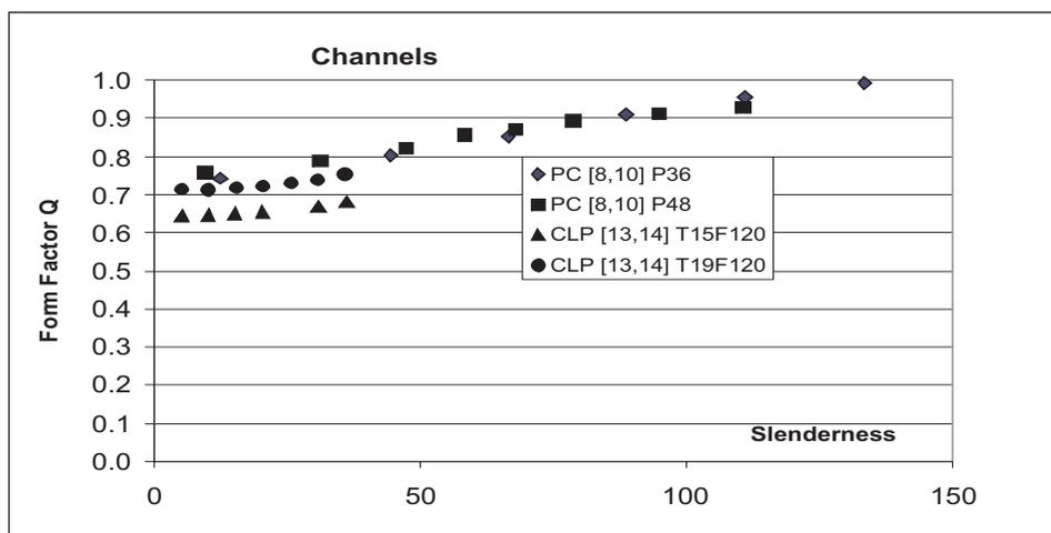
Figure 2 - Form factor versus slenderness for some channels specimens
