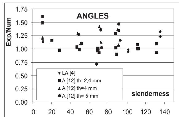
Figure 1 - Accuracy of the method for angles: error versus the specimen slenderness
