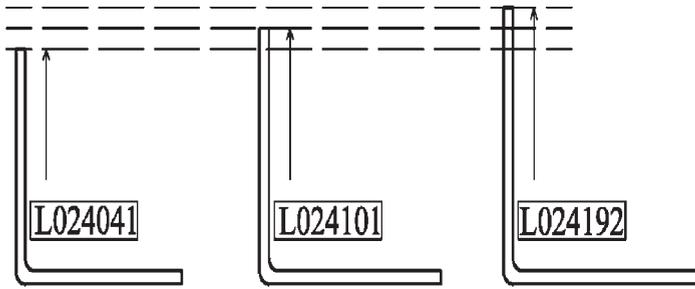
Figure 8: effective section for the considered angle specimens
