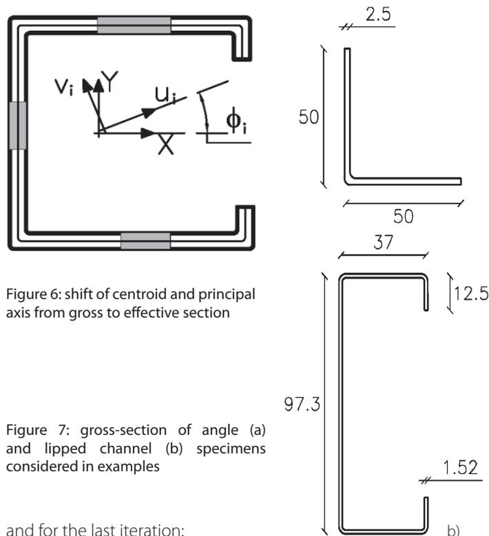
Figure 6: shift of centroid and principal axis from gross to effective section
