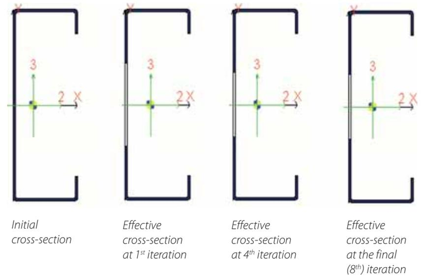
Figure 9: evolution of the effective cross-section for L36F0280 specimen
