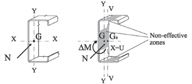
Figure 4: gross and effective cross-section: shift of centroidal axis
