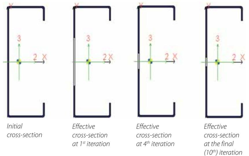
Figure 10: evolution of the effective cross-section for L36F3000 specimen
