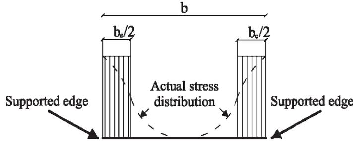
Figure 1: effective width for compressed stiffened element
